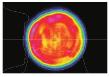
LQ215 laser typical near field beam profile.
