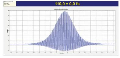
The FX150 laser typical autocorrelation curve.
